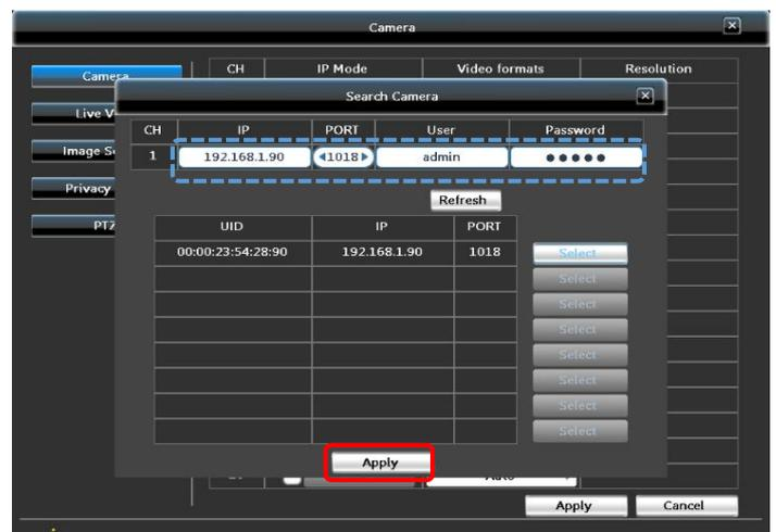
**Step 5.** Go back to the camera page, the selected IP camera applied to the channel already. Click **Apply** and **OK** to save the settings.
