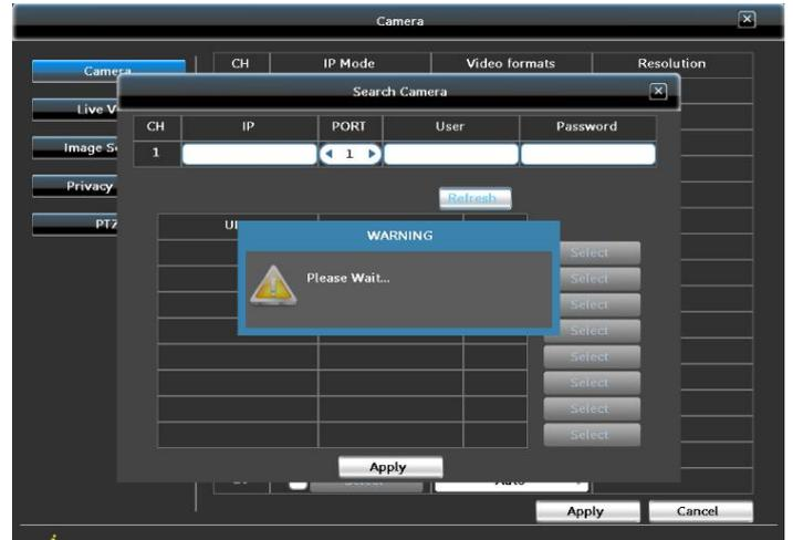
**Step 4.** The IP camera appears in the list, then click the **Select** button. The selected camera will be auto-filled in the upper blanks. Then click **Apply**.
