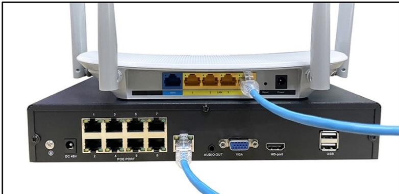
This TIGERSECU NVR also works with third-party branded IP cameras. Connect your IP camera to the NVR PoE port directly if the IP camera is enabled PoE (power over ethernet). If your IP camera doesn't support PoE, connect your IP cameras to the same router/switch with the NVR, so you can add them to your NVR.
