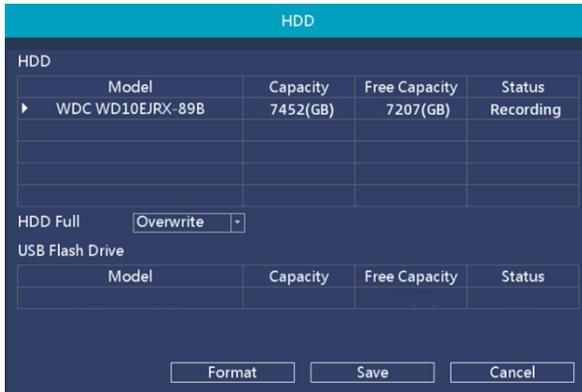
This NVR supports a maximum capacity HDD of 16TB. **CAUTION:** Formatting the HDD deletes all saved files.
