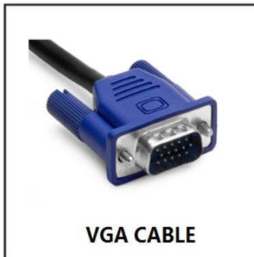
Connect your NVR to a desktop computer monitor or TV screen using a VGA or HD-port cable. The NVR's default display resolution is 1280 x 1024 pixels and will work with TV and desktop computer monitors that support 1280 x 1024 pixels or higher resolution.
