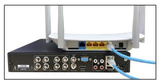
Prepare the DVR, router, and network cable. Connect them as shown in the diagram above.
