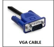
Connect your DVR to a desktop computer monitor or TV monitor using a VGA/HD-port cable. TIGERSECU DVR's default display resolution is 1920x1080 and will work with TV and desktop computer monitors that support 1920x1080 pixels or higher resolution.
